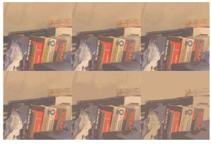
Figure 6. The effects of reducing the number of bits used to display the image. The image in the top left is the starting image. The other two images on the top row are quantized to 8 and 7 bits. The bottom row is 6, 5 and 4 bits from left to right.
